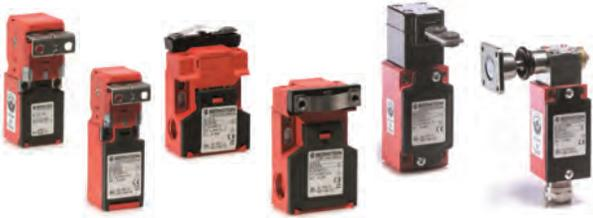
Safety switches with separate keyed actuators provide a failsafe switch function, indicating the position of guarding access points. These are typically used on hard guarding gates, panels and doors. The switches are normally mounted on the fixed frame of the machine. The actuator key mounts on the door. When the door is closed the key is inserted into the switch, closing the normally closed safety contacts.
