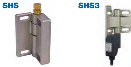
Safety Hinged Switches combine the function of a load bearing hinge with a Category 4 (Ple) rated safety switch. They are easy to install and tamper resistant. Since they do not use an actuation key, there are no alignment or bend radius issues and they cannot be defeated with an extra key. The SHS series is available with 1 NC or 1 Changeover contact. The new SHS3 offers 2 NC/1 NO contacts. Safety Hinged switches are available with the cable attached or with an M12 connector.
