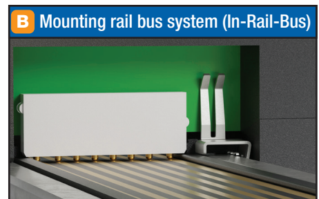
The optionally available mounting rail bus system, In-Rail-Bus, allows for the easy networking of system units by means of a bus PCB integrated into the mounting rail; it is available with 5 or 8 conductor paths.
