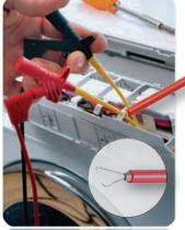
Measuring voltage quickly and easily - this is possible in a wide variety of situations with the units shown on the left. SKS can offer you the clamp-type test probe that you need even special solutions to enable access to difficult-toaccess places. The flexible shaft allows you to connect to wires, pins and eyelets as well as to measuring clamps, and to the finest connections in the electronics field.
