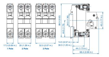
UP 10-13 NOTE When a busbar is used, mixing and matching between the two series is not possible. The terminal positons are different in the Z direction (front to back)
